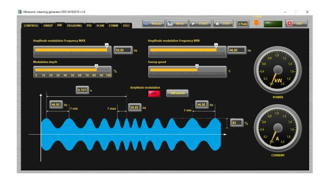
**Amplitude modulation frequency MAX** – This the maximum value of the frequency of the amplitude modulation.
