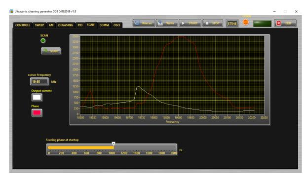
11. Press the SCAN button. The scanning procedure starts. There is a drawing consisting of phase characteristic (red line) and current characteristics (white line). It should be similar to the picture with well-defined phase feature. This diagram shows the actual operating parameters of the transducer. If necessary, pick new Fstart and SPAN (in CONTROL tab).
