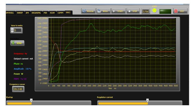
**Startup** – This is the speed of shifting down the operating frequency until reaching Scanning Phase at Startup value.
